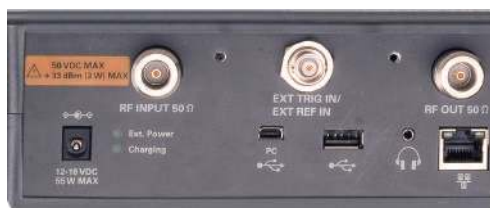
N9340B supports remote control via SCPI over USB and LAN.
